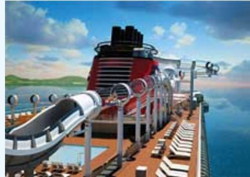
The AquaDuck onboard the Disney Dream, the first water coaster aboard a cruise ship, is 765 feet long, four decks high and swings out over the ocean. Water jets will push guests upwards and forwards at 20 feet per second. Photo courtesy of Disney Cruise Line
